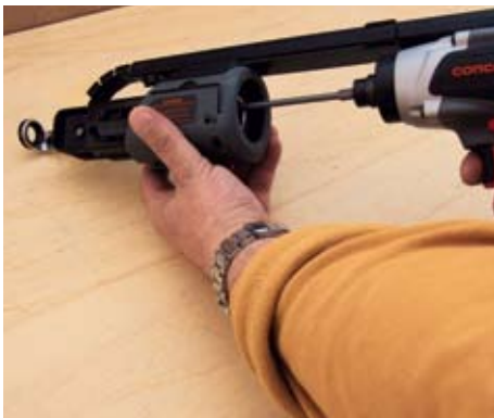
▲ Pic.1 The collated section is easily removed to use the tool as an impact driver
