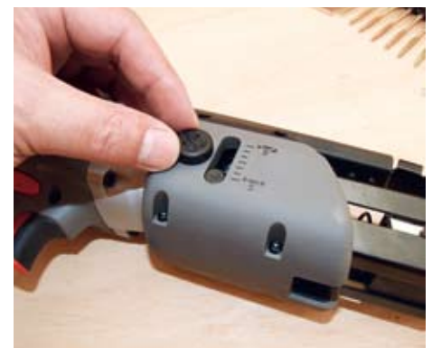
▲ Pic.5 Depth of drive is altered with a simple dial, ensuring consistent positioning
