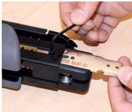
▲ Pic.2 The nose is adjusted with a hex wrench to suit the length of screw being used
